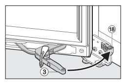
■ Pull the arm of the soft-close mechanism ③ outwards to holder ⑱.
